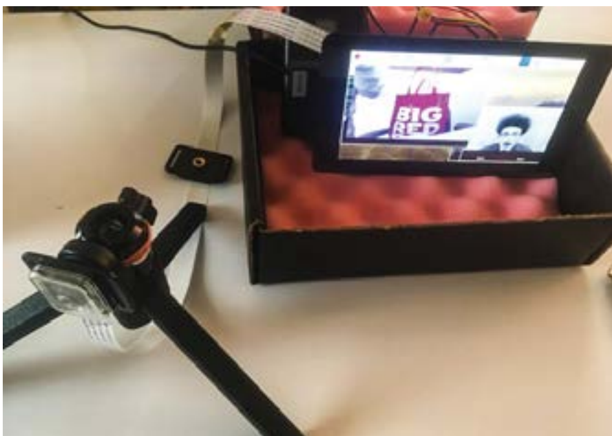
This is the system with the screen face down. That's a Raspberry Pi connected to the little screen; it runs the app and the software that records video and audio. The 'Fifine' USB dongle is the USB connection for the wireless mic. The white cable on the left side goes to the 8 Pixel camera. The white cable on the right goes to the display.
